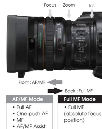
When the focus ring is in the front position, the lens works as an auto focus lens. Either Manual or Auto Focus mode can then be selected using the AF/MF switch on the lens. When the focus ring is set to the back position, the lens has an absolute focus position.
